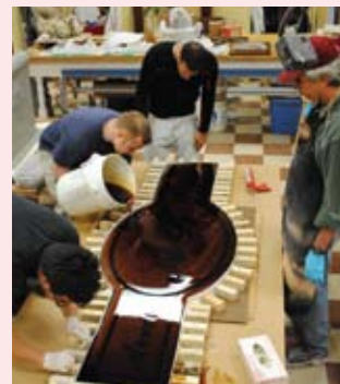
FSU Master Craftsman Studio staff members pouring a mold for the entrance to the Arvah Branch neighborhood.
